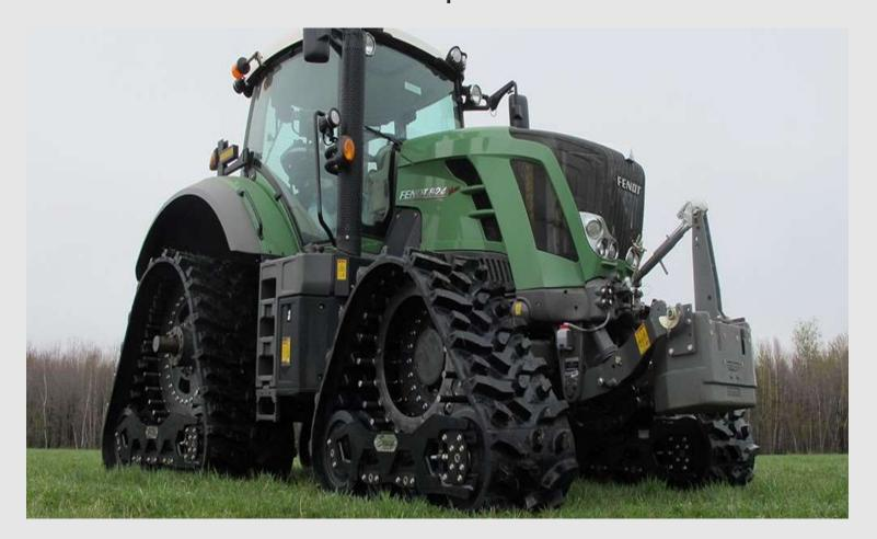
Tyres at low inflation pressure can have an equivalent ground pressure to some track options, however these are wider than tracks and can have a higher draft requirement compared with tracks. Higher purchase and operational cost.
